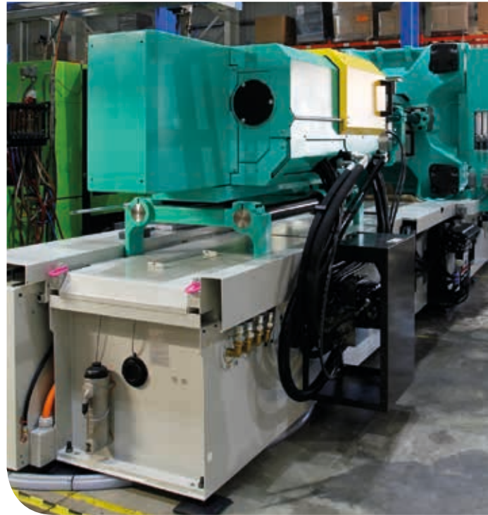
Electrically heated hoses applied in injection-moulding. The liquid plastic must be kept at a constant temperature.
